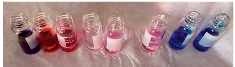
Eight samples with strong color matrices (4 solutions were spiked with 0.2ppb Cr(VI) solution)
